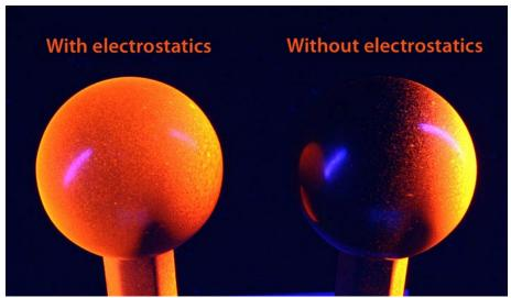
Each was sprayed separately and each spray was the same except for one thing – the left target was sprayed with the electrostatic charging system ON, but the right target was sprayed with the charging system OFF. The results are *astounding*.
